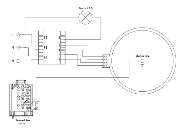
The equipment must be protected by a fused switch. Check the power of the equipment to select correct fuse size (sticker on equipment). An isolator switch also need to be installed. The isolator switch must comply with EU/UK rules and regulations Earth wire must not be isolated via any switch. When installing the equipment make sure during the first operation the wire is not getting warm.
